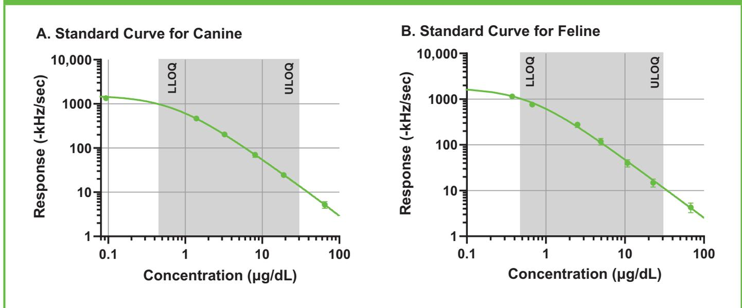
Seven calibrators with known concentrations of tT4 were used to generate a standard curve for (A) canine and (B) feline analysis. The shaded region represents the reported dynamic range. LLOQ, lower limit of quantitation; tT4, total thyroxine; ULOQ, upper limit of quantitation
