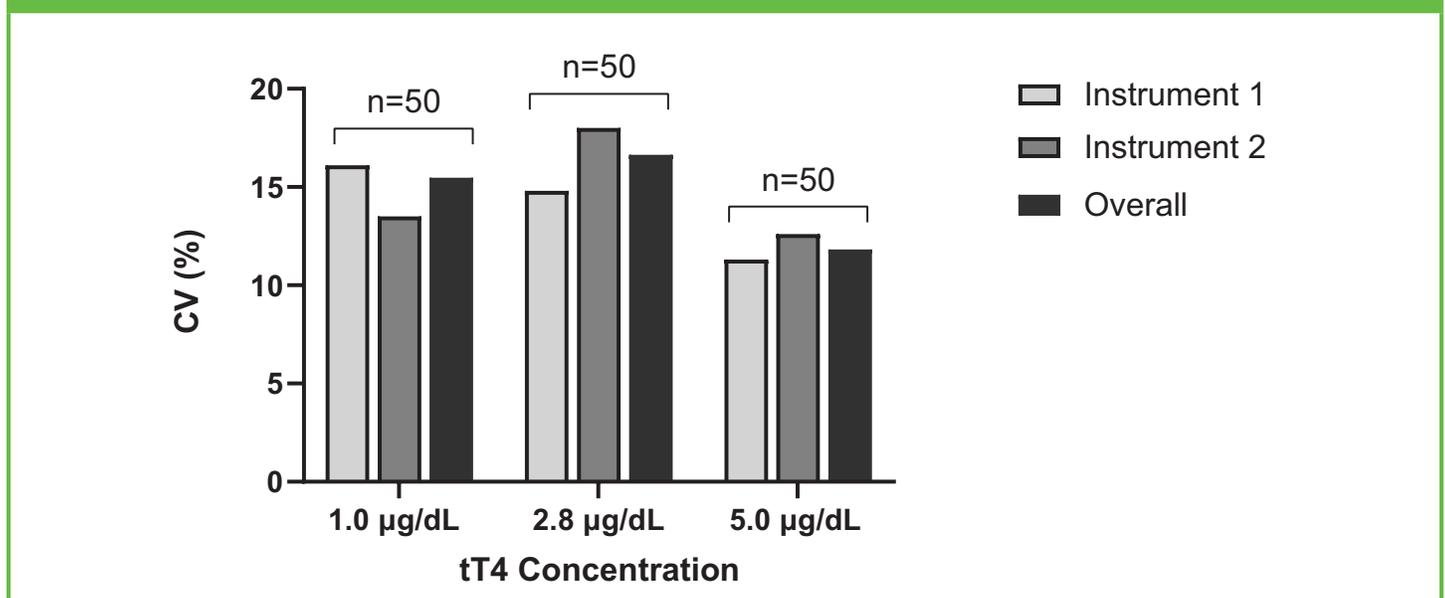
%CV was calculated for three serum samples with varying tT4 concentrations using 150 runs. One statistical outlier was removed from the 5.0 µg/dL data set following CLSI EP05-A3 guidelines. CV, coefficient of variation; tT4, total thyroxine.
